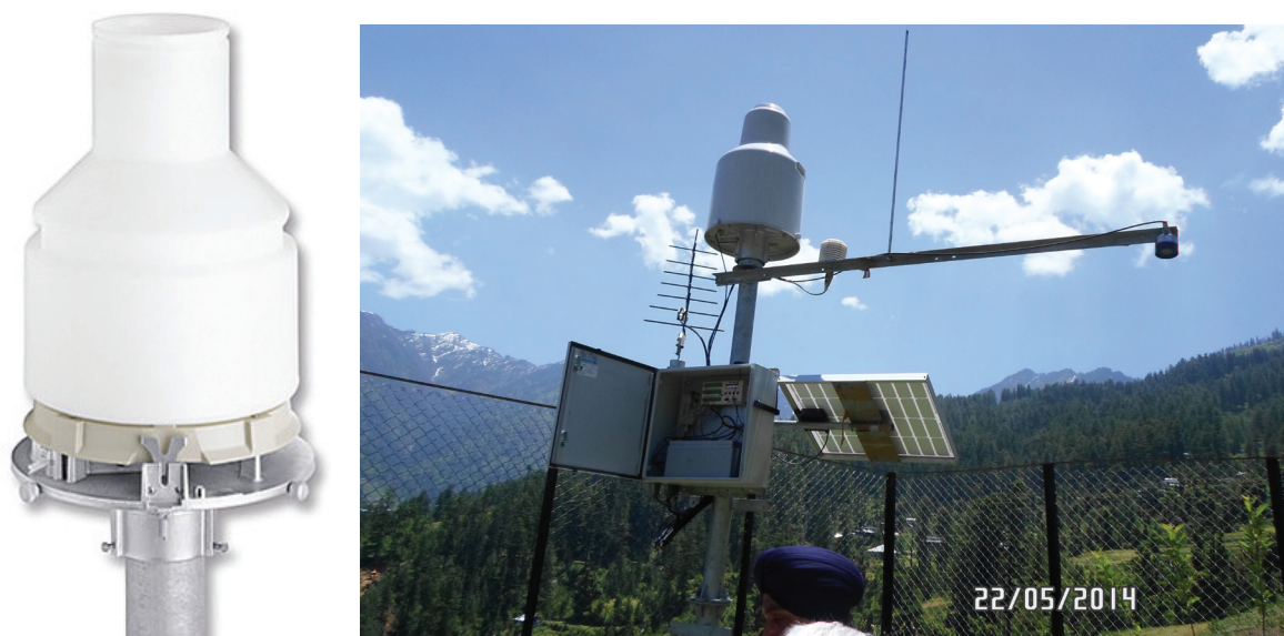
Figure 2.4: Frozen precipitation gauge with 1,000 mm capacity (left). A precipitation gauge installed in Madana, Himachal Pradesh, by Bhakra Beas Management Board (right)
