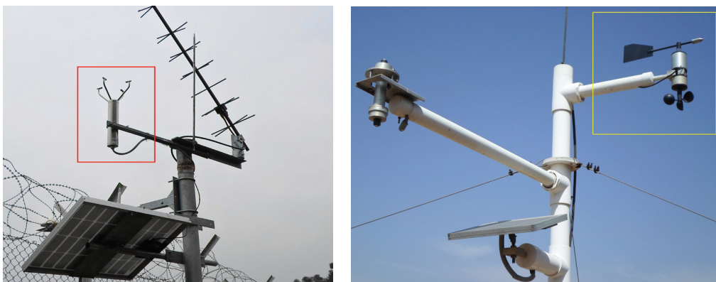
Figure 2.8: An ultrasonic wind velocity and direction sensor (left) and a cup-anemometer and wind vane-based wind velocity and direction sensor (right)
