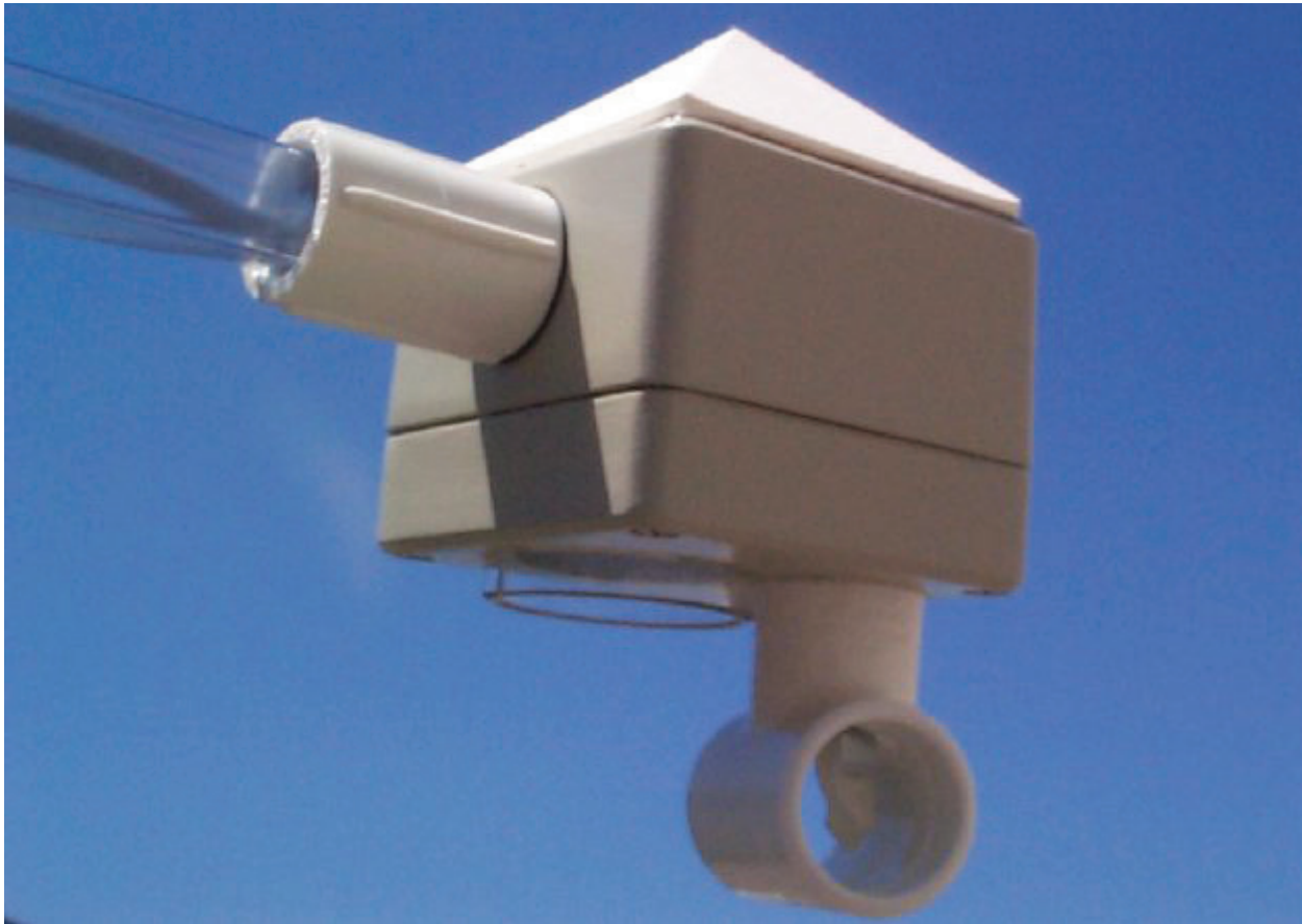
Figure 2.5. A snow depth sensor showing the temperature compensation device on the lower right and the ultrasonic sensor to the left of the temperature compensation device
