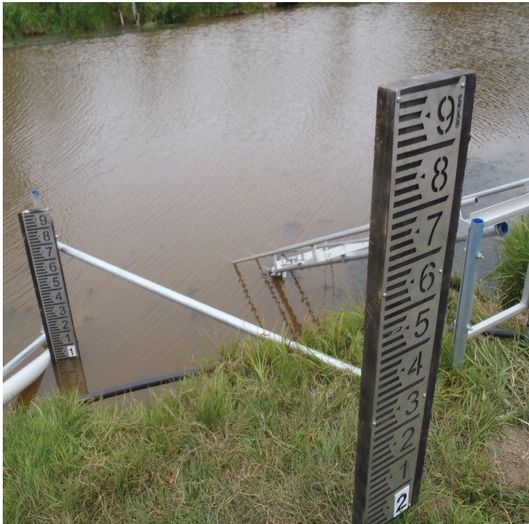
Figure 3.8: A staff gauge in two sections
