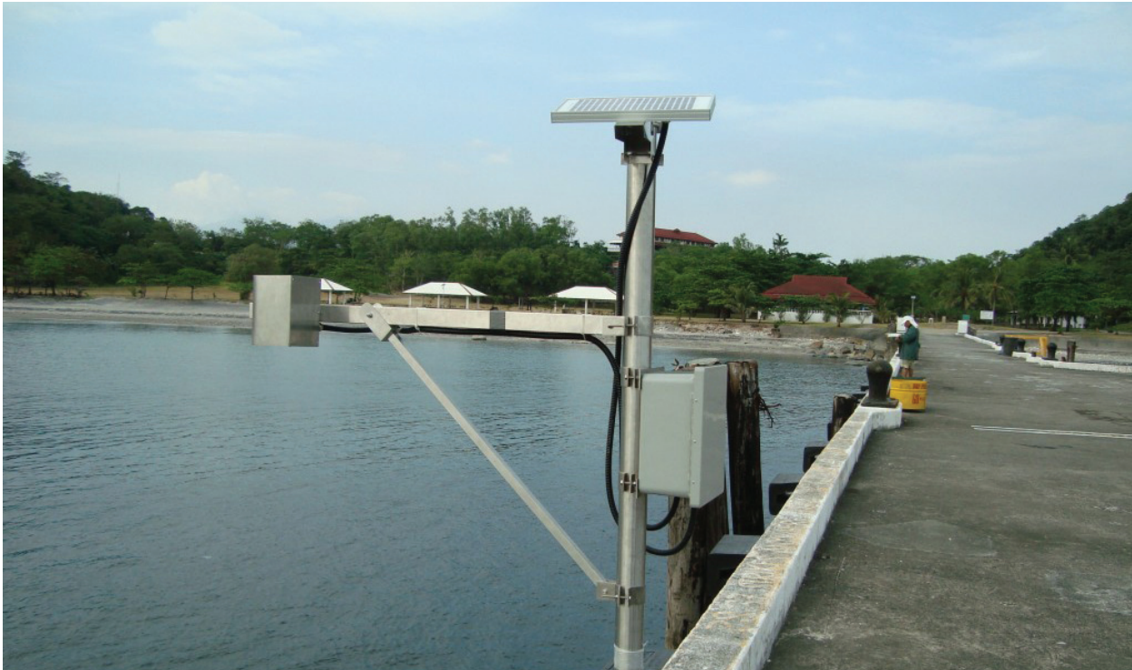
Figure 3.2: An ultrasonic sensor with boom mount
