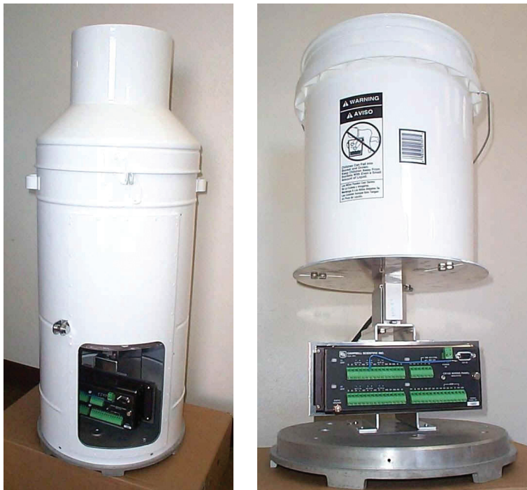
Figure 2.3: Frozen precipitation gauges with 1500 mm capacity
