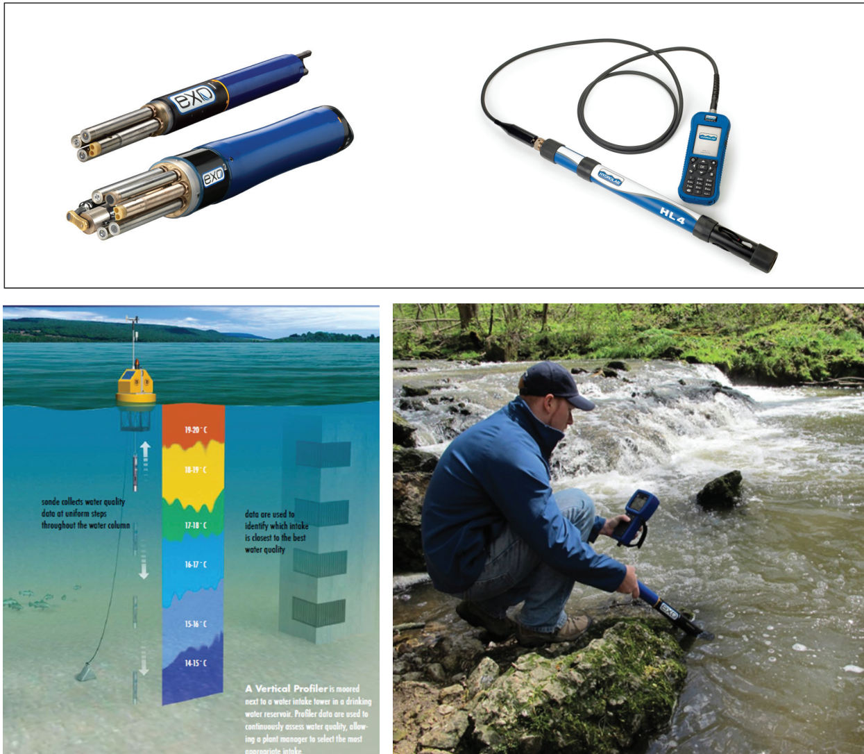
Figure 5.2: A hand-held water quality sampler with a display device (top right); a sampler with multiprobes (top left) ; and measurement options in a stream (bottom left and right)
