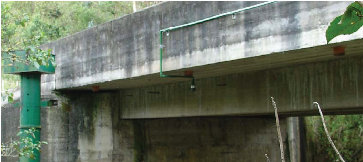
Figure 3.3: An ultrasonic sensor being used to measure water elevation using a bridge mount
