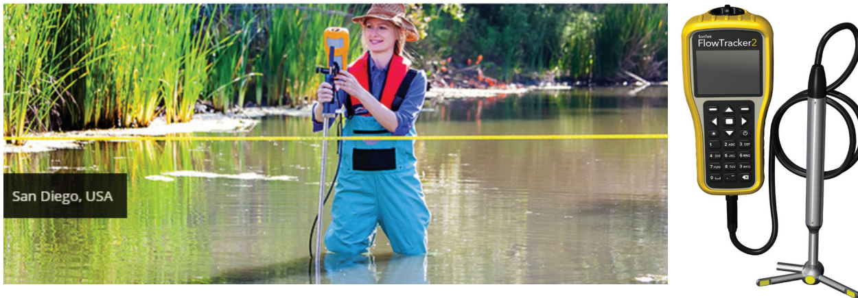
Figure 3.20: A hand-held acoustic Doppler velocity meter
