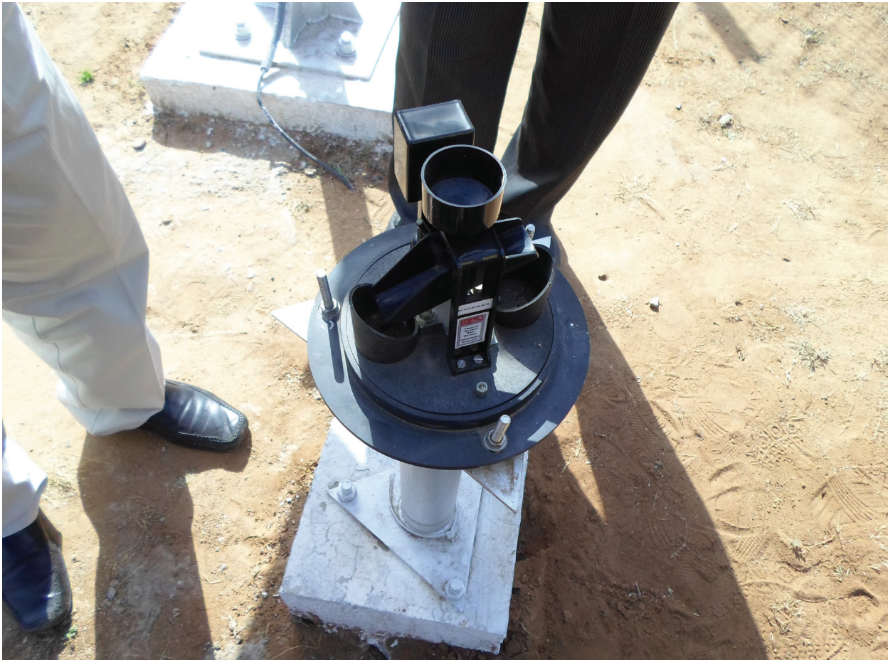
Figure 2.1: A typical tipping bucket rain gauge
